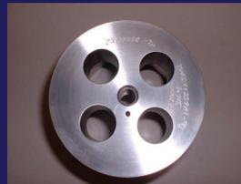
8. Once manufactured, the parts are inspected against the drawing and the work order for material, and dimensional compliance. All parts should be 100% inspected and etched with P/N and Work Order, replicator name, and store code number (if desired)
