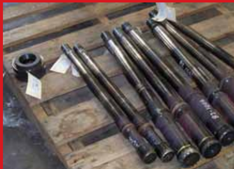
Valtek® 6" Channel Stream Pressure Balanced Plug & Stem Assembly, Multi Stage Retainer and Sleeve
