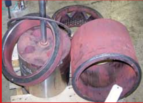
Copes-Vulcan® 12" Plug & Stem, Seat Ring, Cylinder Assemble & Balance Cylinder
