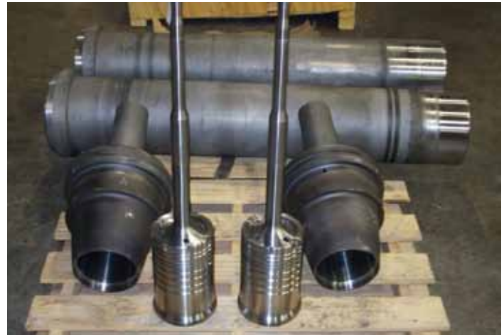
Alstom® High Pressure Spindles, Locks & Seat Chambers
